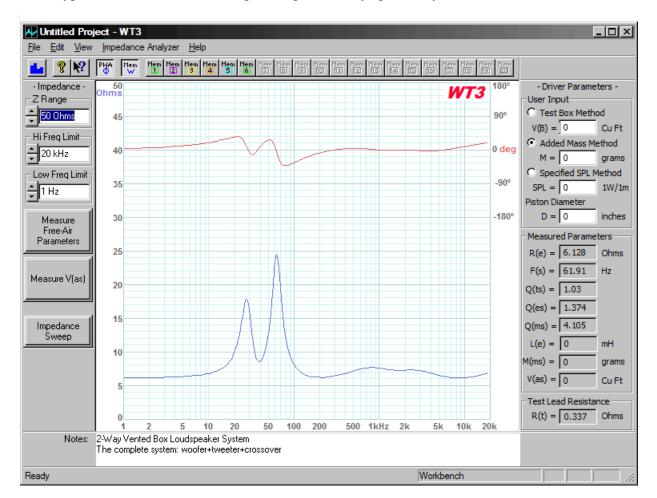
Here is a typical result when measuring a complete 2-way speaker system:
